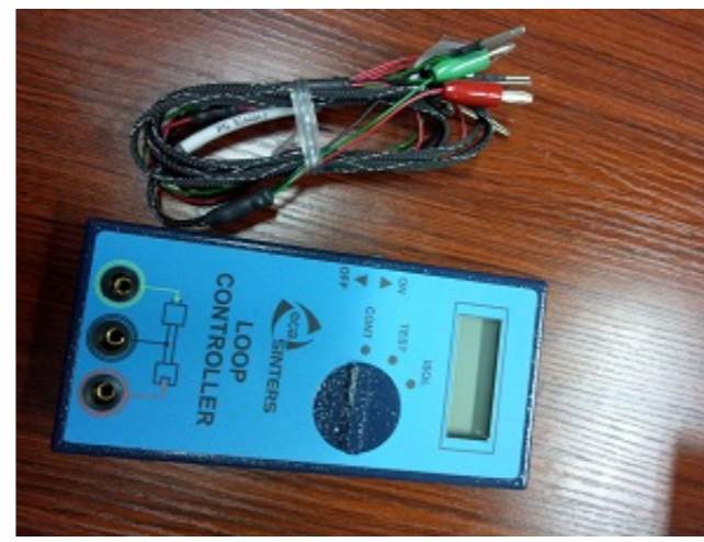
Manual Sinters Loop Controller 9240si
